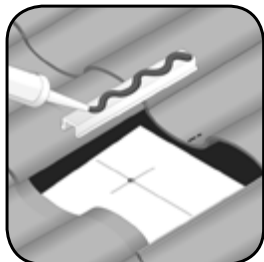
Step 5: Insert the lag bolt and washer through the TileTrac® and apply fresh compatible sealant to the base. Seal tile nail hole.
