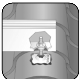
Step 13: Fasten rail with lower and upper 3/8" nuts/washers to 15 ft-lb as shown.
