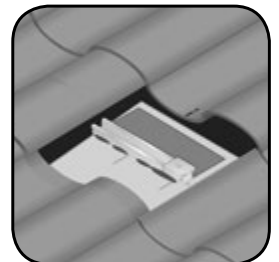
Step 8: After bolting the base to the roof, slide the upper carriage under any portion of the crown (high point) of the tile.* For flat tile, slide the upper carriage near the middle of the tile.*
