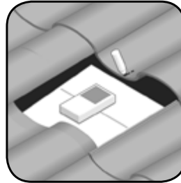
STEP 3: Using an electronic stud finder (recommended), or other means, locate the rafter center. Mark a reference point on the tile above.
